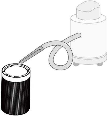
5. If required, replace with a new filter. Unwrap the new filter from the packaging (See page 6 for instructions on how to order a new filter).
