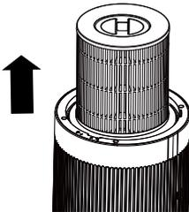
3. The outer surface of the filter should be cleaned every 2–4 weeks to increase the efficiency and extend the life of the filter. Clean the outer surface of the filter using a soft cloth to remove hair, dust, and large particles.
