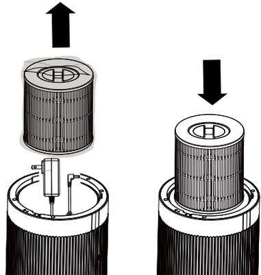
3. Replace the filter cover. Make sure the triangle on the filter cover aligns with the triangle on the bottom edge of the air purifier. Then twist clockwise to lock.
