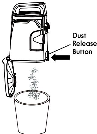
4. Shake the dust cup to release any debris that might hang in the pre-filter.
