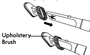
To return the combination tool to crevice tool mode, press the release button and slide the brush tool down the combination tool.
