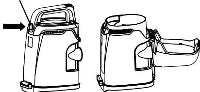
3. Clean pre-filter by gently tapping over a trash container. Tap on several sides to ensure best cleaning.
