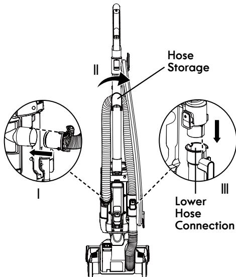
6. Store the extension wand under the hose storage as shown. Make sure the smaller end of the extension wand is upward. Push and snap into place.
