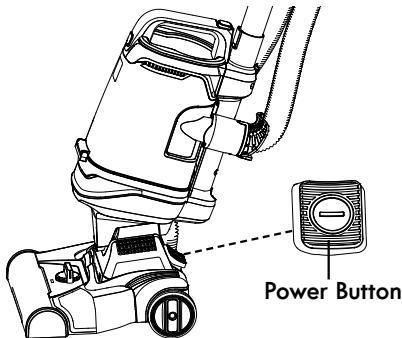
3. Once the vacuum is on, operate the vacuum cleaner by tilting the handle back towards you and the nozzle is flush with floor surface.
