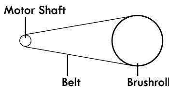
8. Reinstall the brushroll back into the floor nozzle by placing end caps into slots. First align the end cap of belt side of the brushroll with the slot and insert it into place. Then press down the end cap of the non-belt side firmly into the slot as shown below. Rotate the brushroll to make sure the belt is installed correctly.
