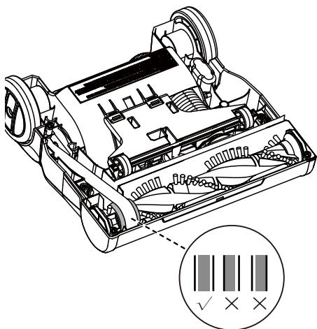
9. Reinstall the lower plate by aligning tabs on front edge of lower plate with slots in the nozzle first, and then press the lower plate to installed position.
