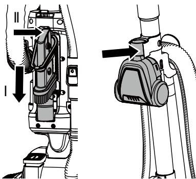
8. Make sure the upper cord hook is in the proper position as shown. Wrap the power cord loosely around the upper and lower cord hooks.
