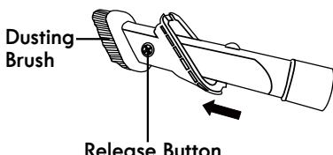
Press the release button to remove the brush tool. Set the combination tool in upholstery brush mode as shown. Use in upholstery
