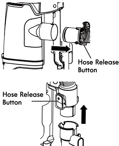
3. Check and remove any clogs in the flexible hose.
