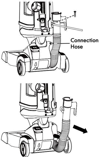
3. Reinstall the collection hose and fix with the screw. Do not over-tighten the screw.
