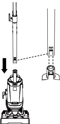
3. Align the attachment holder clip with the front of the wand as shown. Make sure the oval hole aligns with the corresponding protrusion on the wand. Push and snap into place on wand.
