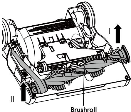
5. Remove the worn or broken belt.
