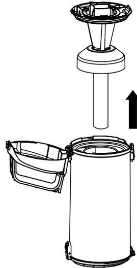
4. Clean pre-filter by gently tapping over a trash container. Tap on several sides to ensure best cleaning.
