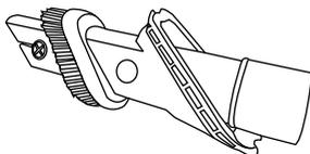
Set the combination tool in dusting brush mode by pressing the release button and sliding the dusting brush side of the brush tool to the end of the combination tool. Use in dusting brush mode for cleaning loose surfaces such as drapes. See ATTACHMENT USE TABLE (page 13).
