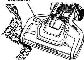
**To correct problem:** Turn off and unplug the vacuum cleaner, remove obstruction, then turn on the vacuum cleaner.
