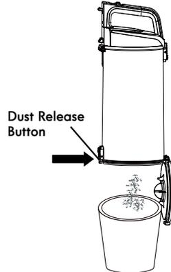
4. Shake the dust cup to release any debris that might hang in the pre-filter.
