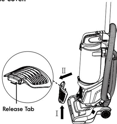
2. Remove the HEPA media exhaust filter from vacuum cleaner.
