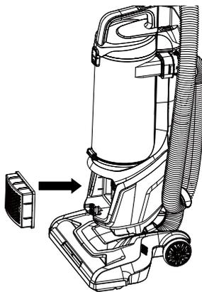
5. Insert the exhaust filter cover tabs into the upper slots and lock the filter cover into place by pressing the lower part of the cover until a click is heard.
