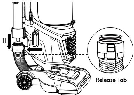
2. Check and remove any clogs in the hose.
