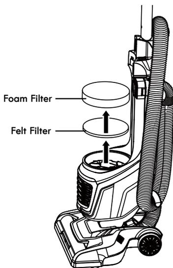
3. Wash with cold water only, **DO NOT** use detergent or soap. Squeeze by hand and allow to air dry. Allow all filters to dry 24 hours before putting back into vacuum cleaner.
