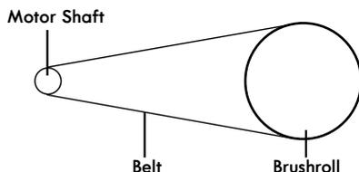
7. Reinstall the brushroll back into nozzle by placing end caps into slots. First align the end cap of non-belt side of the brushroll with the slot and insert it into place. Then press down the end cap of the belt side firmly into the slot until a click is heard. Check the brushroll to ensure it rotates smoothly.
