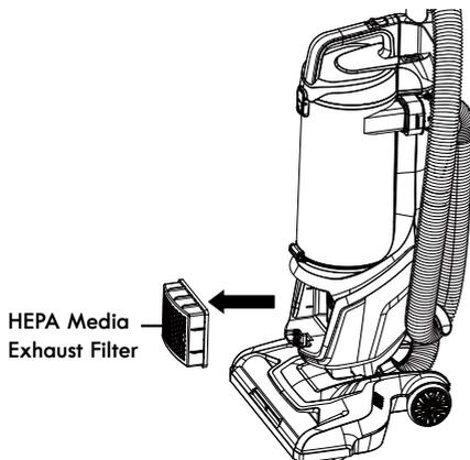
3. Wash with cold water only, DO NOT use detergent or soap. Allow to air dry. Allow parts to dry 24 hours before putting back into vacuum cleaner.
