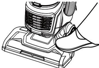
2. Turn on the vacuum cleaner by pressing the On/Off switch to the "I" position for cleaning bare floors and small area rugs.
