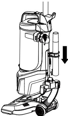
3. Insert the end of the flexible hose into the main body by aligning marks as shown in UNLOCKED (for cleaning). Rotate the hose until marks align as shown in LOCKED (for use). Then run the flexible hose over the lower hose storage and the upper hose storage. Insert the other end onto the top of the extension wand.
