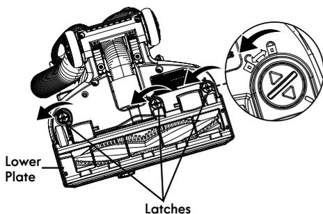
3. Remove the brushroll by carefully lifting it out.
