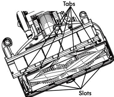
9. Press the lower plate onto nozzle until a click is heard and secure by rotating the lower plate latches clockwise to the LOCK position.
