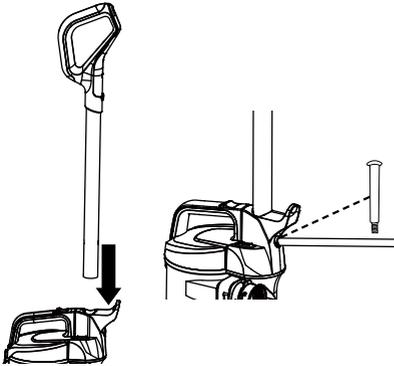
2. Insert the larger end of the extension wand into the top of the connection hose through the bracket until the wand is fully seated on the post.
