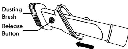
Press the release button to remove the brush tool. Set the combination tool in upholstery brush mode as shown. Use in upholstery brush mode for cleaning fabric surfaces such as fabric sofa. See
