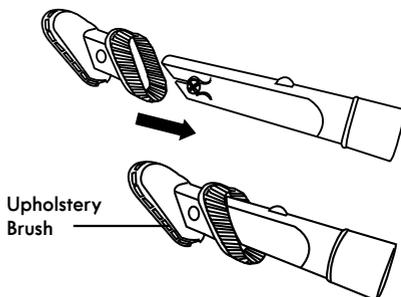
To return the combination tool to crevice tool mode, press the release button and slide the brush tool down the combination tool.
