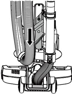
5. Make sure the upper and lower cord hooks are in the proper position as shown. Wrap the power cord loosely around the upper and lower cord hooks.
