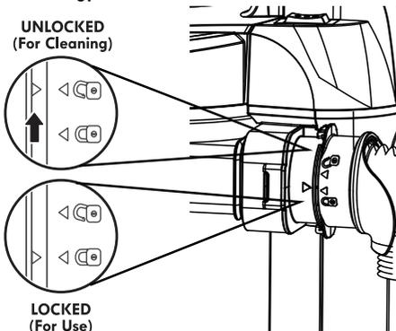
3. Remove hose end, check and remove any clogs in the flexible hose.
