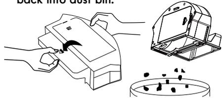
3. Open the filter cover and take out the filter and filter basket.
